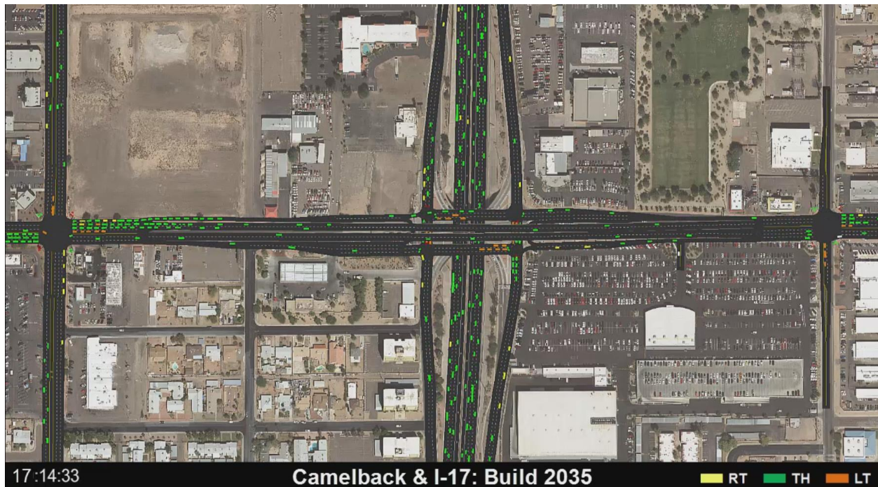
FIGURE 10 An aerial view of the 2D animations of the 3-level platform at Camelback Road and I-17
